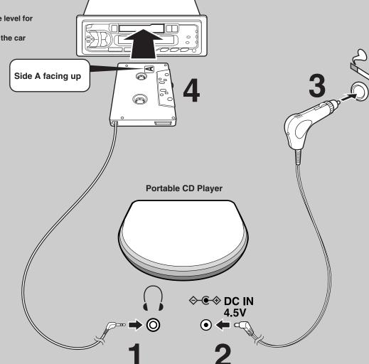
If the position of the cord coming out of the cassette adapter is adjusted using the groove provided on the back of the cassette, it will work with almost all car audio systems:
